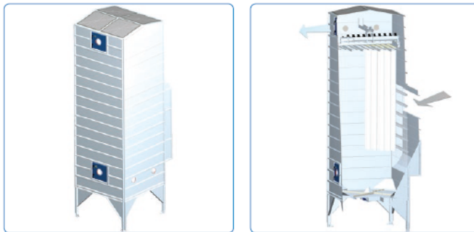
Figure 5. View and section through a SuperJet filter [10].
