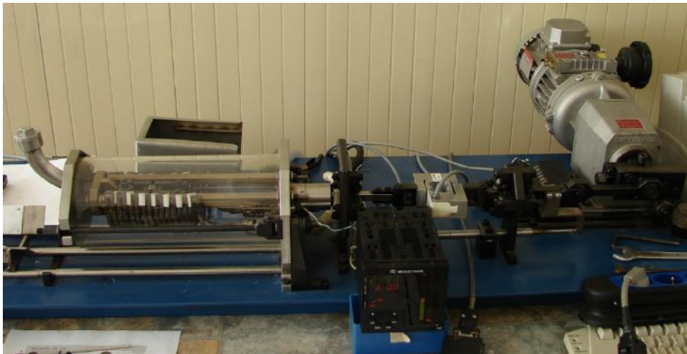
Figure 1. The equipment used for simulated power cycling fatigue
