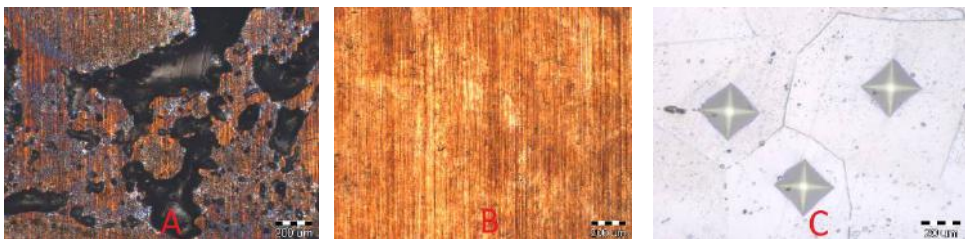
Figure 17. Specimen 9 A) covered with lead B) after cleaning test at 75 °C in Sol. 3 C) Vickers microhardness after cleaning test
